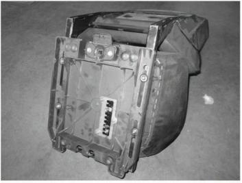
1. Remove stock seat from vehicle by reaching behind seat and pulling on the release handle [RED].
