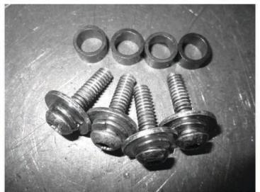
4. Separate the spacers from the bolts, as you will not be using the spacers for the Proarmor seat installation. Retain both the lock washer and flat washer.
