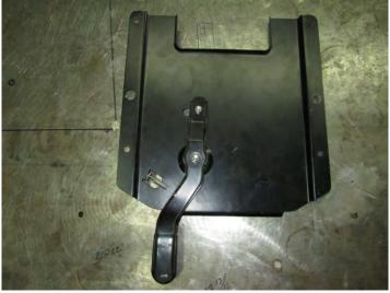
5. Remove the (4) T27 Torx bolts holding the seat cushion and stock seat slider to the seat frame [GREEN]. Set this hardware aside, as you will not use it for the remainder of this install. Refer to the following two diagrams on the next pages to disassemble the stock seat slider and assemble your new Proarmor seat slider.
