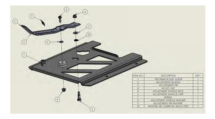
A. Use a 10mm socket to fasten the nyloc nut and either an 8mm socket or T30 Torx bit to fasten the adjustment handle bolt.
