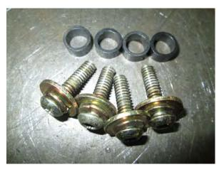
A. Gather the mounting hardware shown. You can put a small amount of blue Loctite 242 on the bolt threads. This will ensure that they will not loosen due to repeated seating position adjustment.
