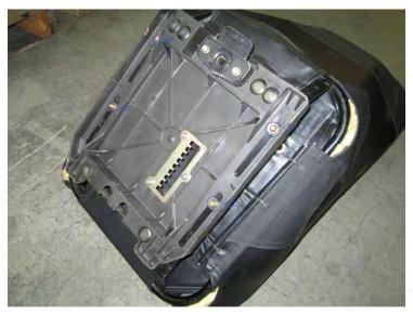
A. Proarmor Pro-Am and Sniper seats have an integrated release strap built into the rear of the seat. If you have a Pro-Am or Sniper seat, you will need to remove the release strap from the release handle on the stock seat base by removing the (2) Phillips head screws [RED].
