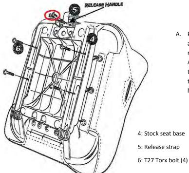
A. Proarmor Pro-Am and Sniper seats have an integrated release strap built into the rear of the seat. If you purchased a Pro-Am or Sniper seat, you will need to install the release strap to the release handle on the stock seat base using the (2) Phillips head screws you removed earlier [RED].
