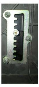
7. Now, you will attach the assembled Proarmor seat slider to the plastic seat base. To do this, pull on the adjustment handle as you set the seat slider onto the plastic seat base. Make sure the seat slider is aligned properly on the seat base and that the adjustment pin can engage each notch on the selection plate. Improper alignment may prevent the slider from moving smoothly on the base.
