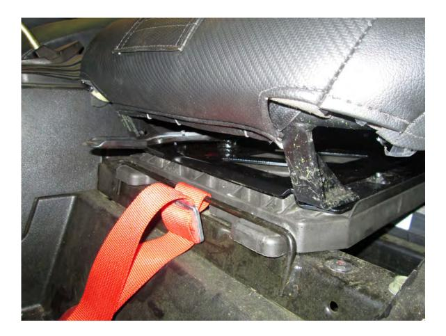
10. Place the seat assembly back into the vehicle. Make sure the seat base "clicks" into place. Test the seat slider functionality and see that you can slide the seat forward and back smoothly and with ease. If there is any binding or it is difficult to slide the seat, double check to make sure the seat slider is mounted properly on the seat base and that you did not overtighten the mounting hardware. Once you are satisfied, installation is complete.
