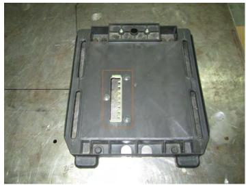
3. Remove the plastic seat base by pulling on the seat position adjustment handle, so that the adjustment pin clears the notches in the selection plate [ORANGE] integrated into the plastic seat base. Then, lift up and away from the bottom of the seat. Proceed to step 5.
