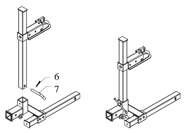
NOTE: In some cases the coupler comes with a bolt installed for shipping purposes only. This must be removed before the unit will operate properly! Be sure to adjust the coupler nut to the hitch ball size before operation!!!!
