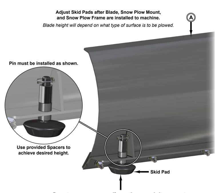
Premature wear may occur if operating on asphalt or concrete.
