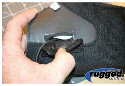
**STEP 5:** You'll notice the hole where the chin strap goes through on the cheekpad. On the velcro side, you can access the inside of the cheekpad. Fold down the fabric as shown in the picture above, and work the speaker into the inside of the padding. Be sure to insert the speaker so that it's facing the right direction, towards your ear. Notice on the picture how the foam is not between the speaker and where your ear will be.
