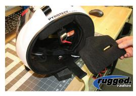
**STEP 4:** That makes the install a little bit faster and easier but we'll show you what to do here if you have a Pyrotect that doesn't have that "pocket". Start by removing the cheek pad that's velcroed to the shell. We start with the one that's not going to have the mic boom on that side.
