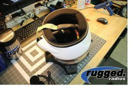
**STEP 2:** Find some way of propping the helmet upside-down. The helmet will be like this throughout the install and propping it this way will stop it from rolling away while working on it.
