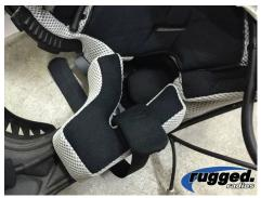
**STEP 3:** Some helmets, like this bisected Motocross style helmet above, have a little pocket for your ear that allows you to simply stick the velcro patch onto the shell, and apply the helmet speaker.
