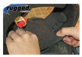
STEP 14: You will need to hold the mic boom securely in place until the hot glue has cooled and cured. Now that the mic boom isn't going anywhere, you can reattach the cheek pad to the helmet over the mic boom. You may need to push the pad firmly against the shell to get the velcro to stick since the boom is between them now. The pad will contour itself around the boom, and will stay securely inside the helmet.
