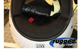
**STEP 7:** The cable that goes from one speaker to the other will need to be secured somewhere in your helmet. The best place on this helmet is along the rear pad that runs along the back of your neck. Begin pushing the wire down between the padding and the shell of the helmet, just enough to get it started.
