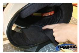
**STEP 6:** This picture simply shows me making sure the speaker is where the wearers ear will be inside the helmet. This would be a good time to put the helmet on see if the speaker needs to be adjusted. If everything checks out, reattach the cheek pad and you're good to move on.
