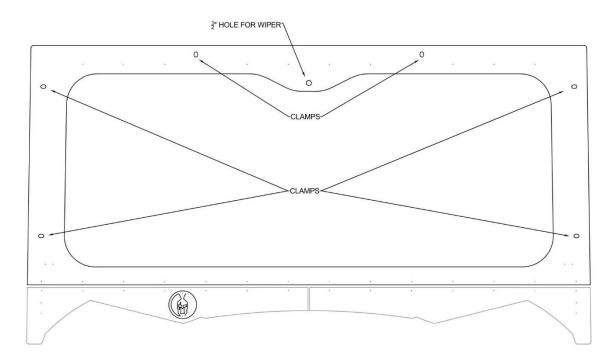
This is just an example of one of our windshields and clamp placement. Each windshield model has different characteristics and clamp placement. In general, this is just a guide.
