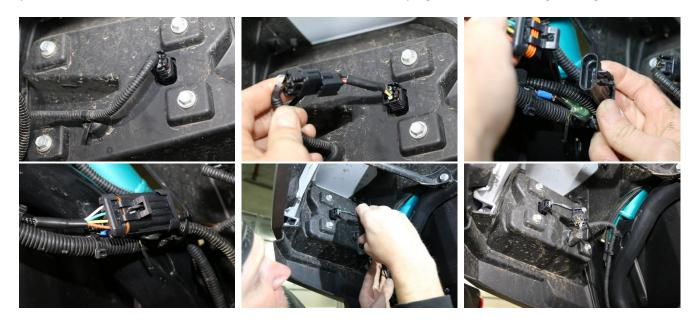
4. Unroll the long extension cable and plug it into the 4-way connector that was just installed from the 4-pin connector down to the rear fire wall through the rubber grommet with the other cables behind the driver's seat, go across to the center console and run alongside the shifter up to the control module that was installed in step 2 and plug in. Keep it away from any **HOT or MOVING** parts. Using the provided Cable Ties secure it to the main OEM wire harness
