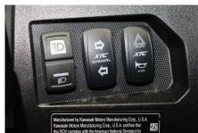
**Dielectric Grease** - Just like the OEM uses on their switches, we recommend using Dielectric Grease on all switch terminals, this keeps the water out, thereby reducing corrosion and helps increase reliability! Open the grease and put on the switch terminals and the connector terminals on both the Turn and Horn switches, the more the better.
