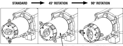
Note: Motor casing rotates with End Cap
