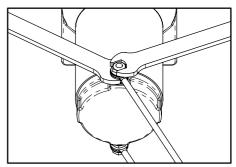
Proper Terminal Tightening
