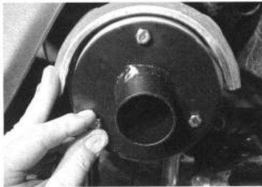
Install Adapter-Tighten Bolts Evenly- Let Silicone Dry- Recheck Bolts After Running
