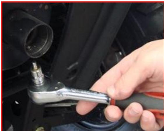
Remove the existing hex bolt from the OEM muffler as shown.
