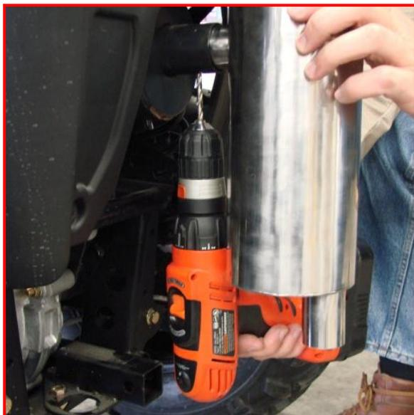
Next, drill back through the stealth and replace the self tapping OEM Bolt to secure the Stealth.
