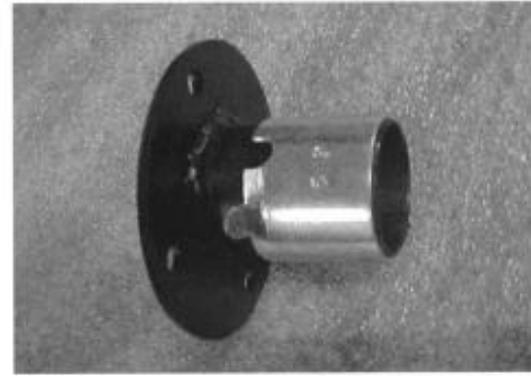
To use elbow adapter, slide #59 split bushing adapter on to outlet as shown. This makes 1 1/2" O.D. needed for elbow. Use sealant
