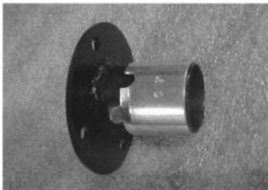
To use elbow adapter, slide #59 bushing onto the outlet as shown. This make it 1 1/2" O.D. needed for use with elbow. Use sealant.
