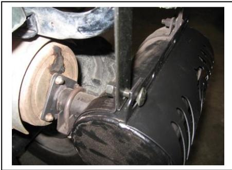
2. The Kolpin Heat Shield has three slots (top and bottom) to make it easier to center the shield over the muffler, no matter what position your muffler is located. (1)
