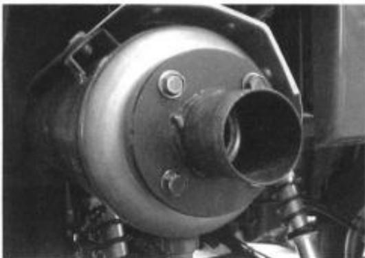
Bolt adapter in place. For direct installation – muffler will slide directly over this adapter. Use 1 3/8" muffler clamp.
