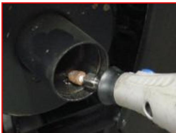
Grind the access material sticking up inside the tailpipe from where the existing bolt was threaded. This allows the Kolpin Muffler to slide in easily.
