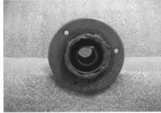
Apply HI-TEMP Silicone to Both Side of Gasket and Install in Place
