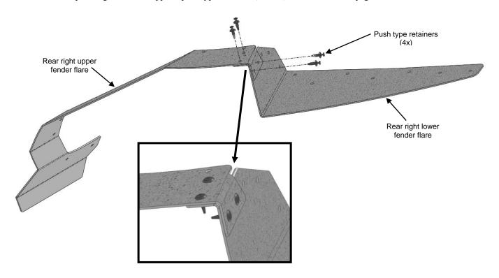
g) Attach the rear right fender flare assembly to the OEM fender using the OEM push type retainer removed in previous step e) and temporarily secure the remaining section of the rear right fender flare assembly to the vehicle using spring clamps or any other clamping tools as shown below.
