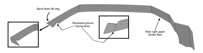
• Assemble both parts together with supplied push type retainers (Item G) as shown on next page.
