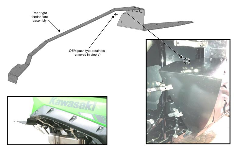
h) Ensure that the rear right fender flare assembly is in proper position and use the remaining mounting holes (20x) as guide to drill <sup>5</sup>/<sub>16</sub> inch diameter holes through the vehicle rear fender and secure right away with the supplied push type retainers as shown below.
