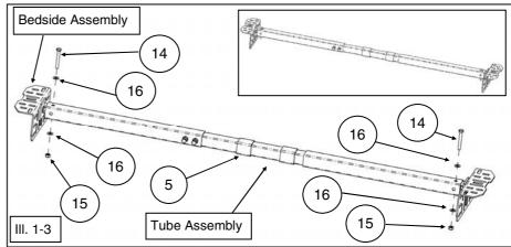
Position the Stronghold Adjustment brackets (item #1) onto the tube assembly. Insert the long M8 bolts (item #14) thru the holes in the adjustment bracket (item #1)
